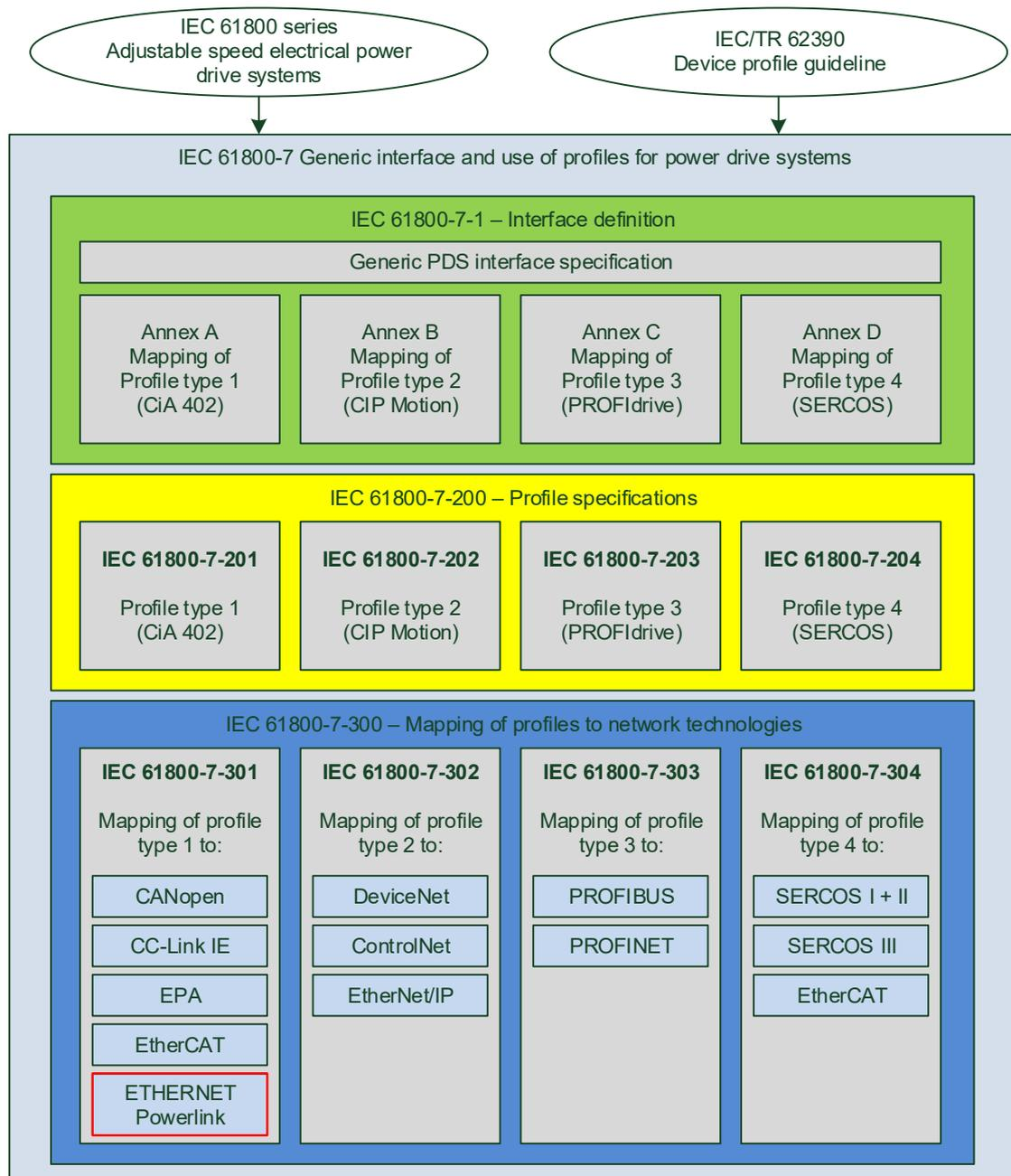
Figure 1: Structure of the IEC 61800-7
