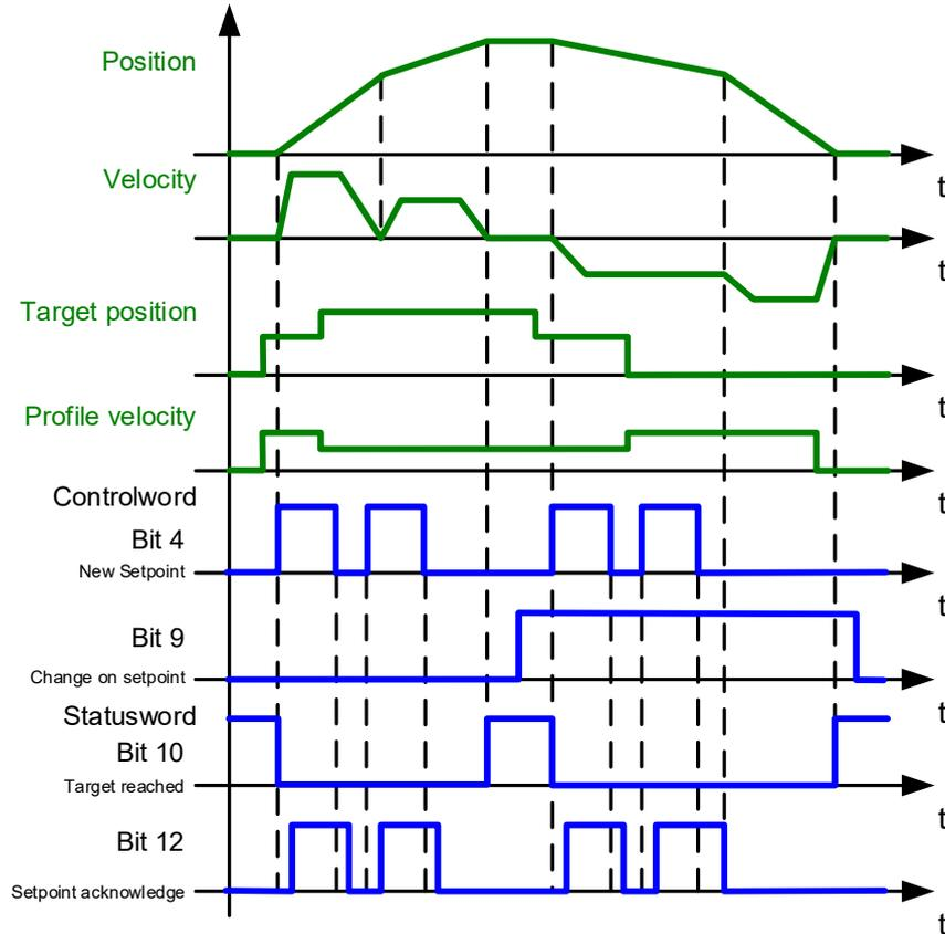
Figure 12: Handshaking procedure for the set of set-points method
