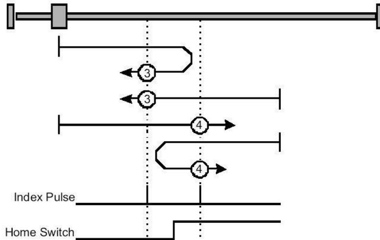
Figure 31: Homing on the positive home switch and index pulse
