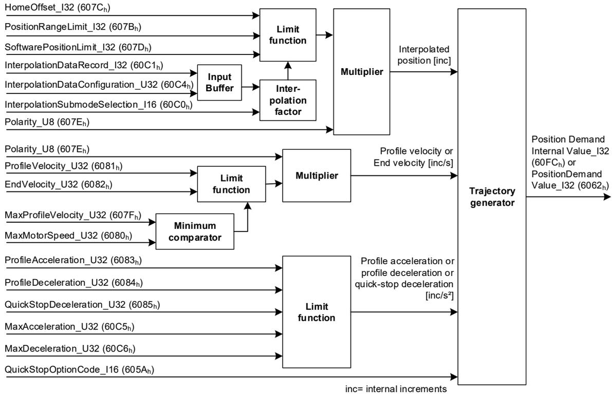
Figure 19: Interpolation controller
