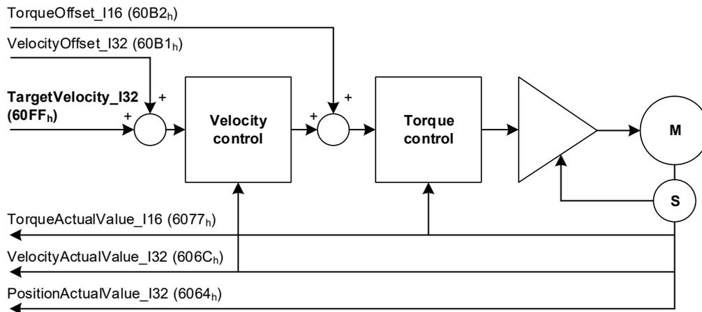
Figure 24: Cyclic synchronous velocity mode overview
