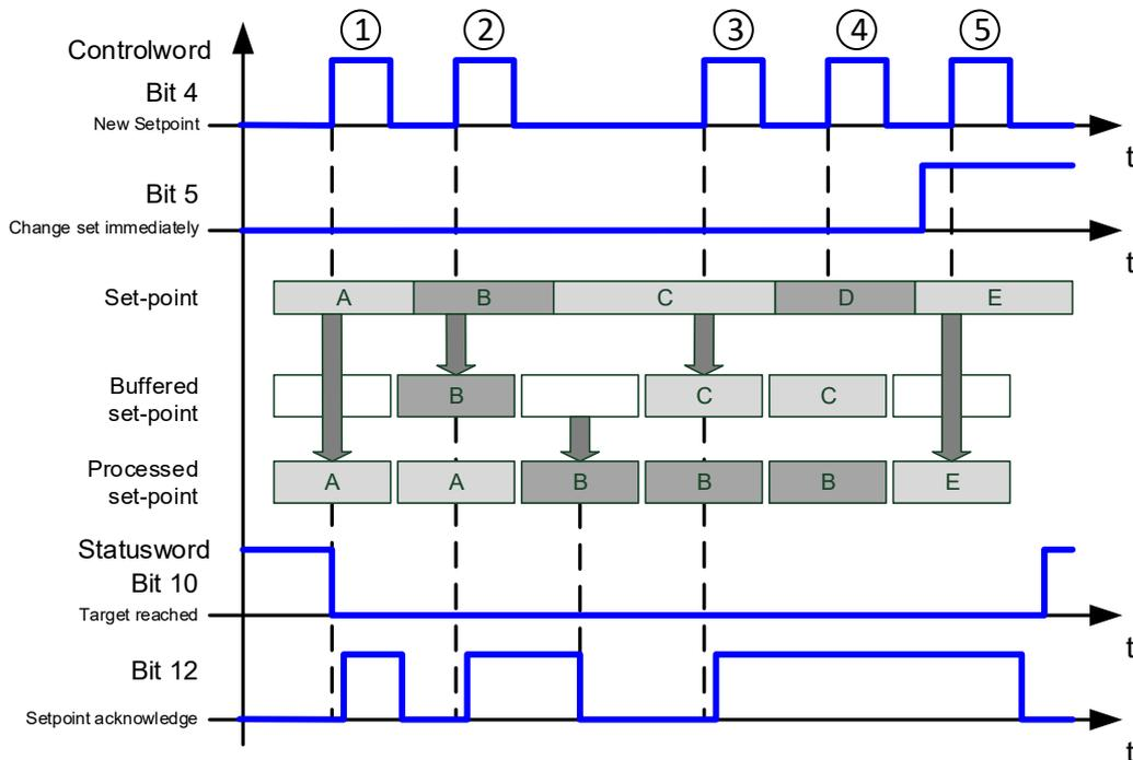
Figure 13: Set-point handling for two set-points
