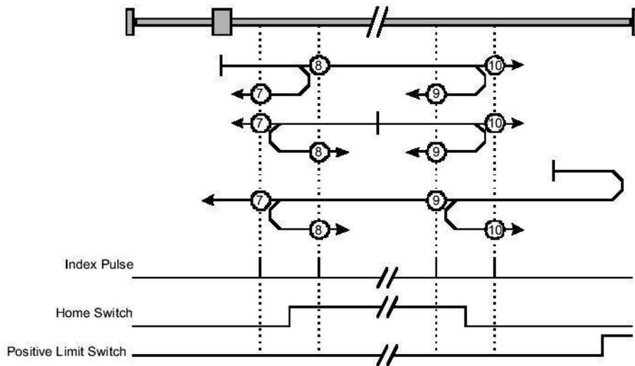
Figure 33: Homing on the home switch and index pulse — positive initial move
