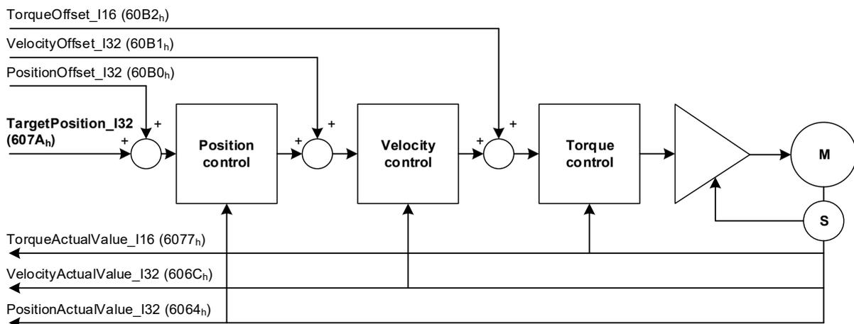
Figure 22: Cyclic synchronous position mode overview
