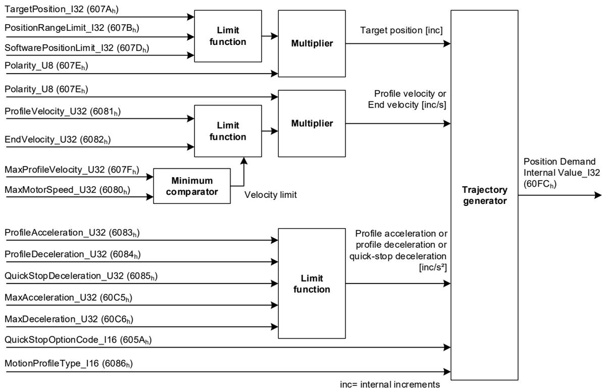
Figure 9: Trajectory generator for profile position mode
