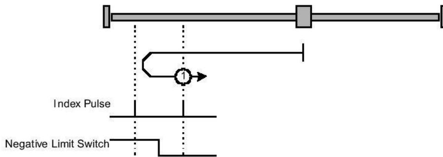
Figure 29: Homing on the negative limit switch and index pulse
