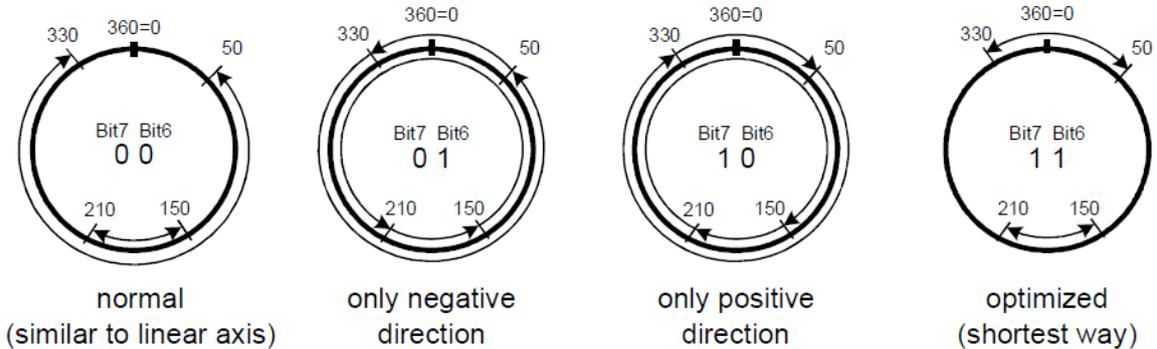
Figure 39: Rotary axis positioning
