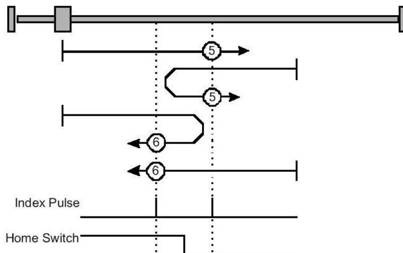
Figure 32: Homing on the negative home switch and index pulse
