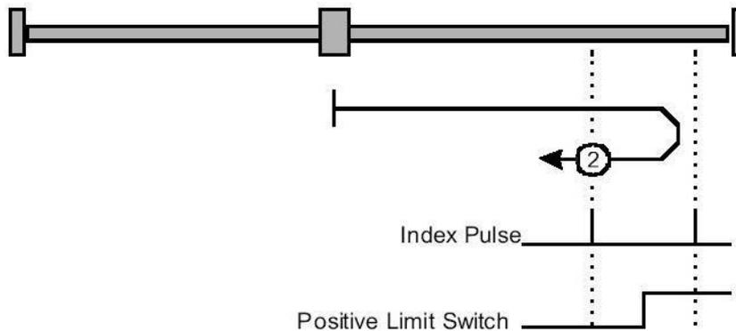
Figure 30: Homing on the positive limit switch and index pulse
