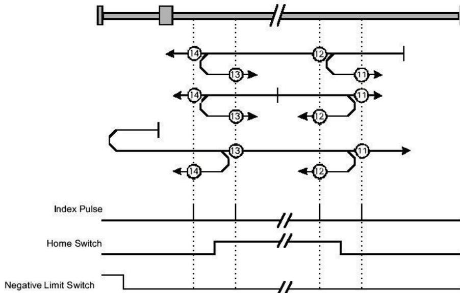
Figure 34: Homing on the home switch and index pulse — negative initial move
