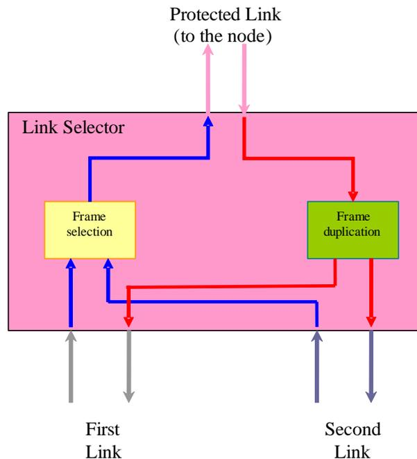
Fig. 2. Link Selector functional block
