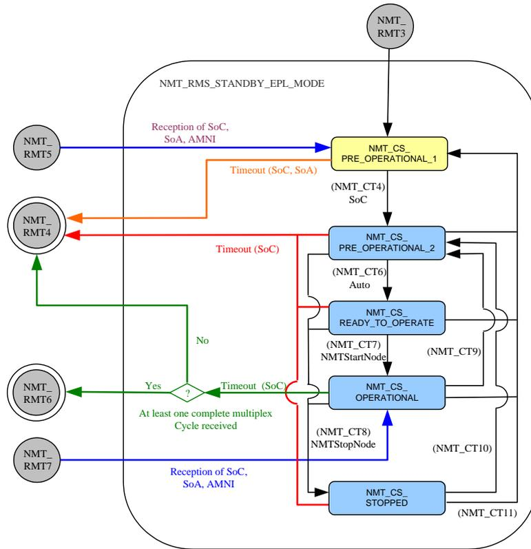
Fig. 17. Detail state NMT\_RMS\_STANDBY\_EPL\_MODE
