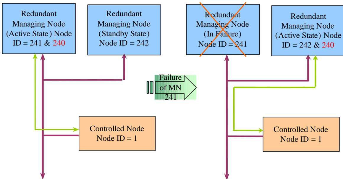
Fig. 6. Flying "240" Node-Id on failure of Active MN
