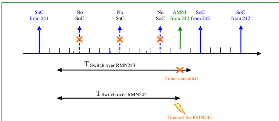
Fig. 20. Example of switch-over with configured large priorities
