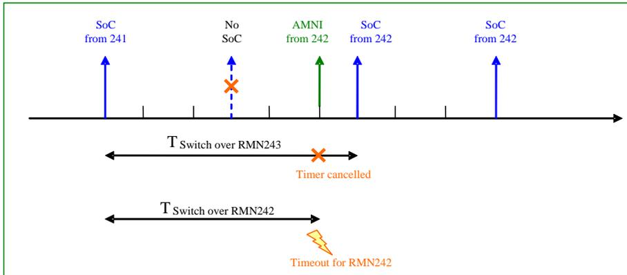
Fig. 19. Example of switch-over with configured priorities
