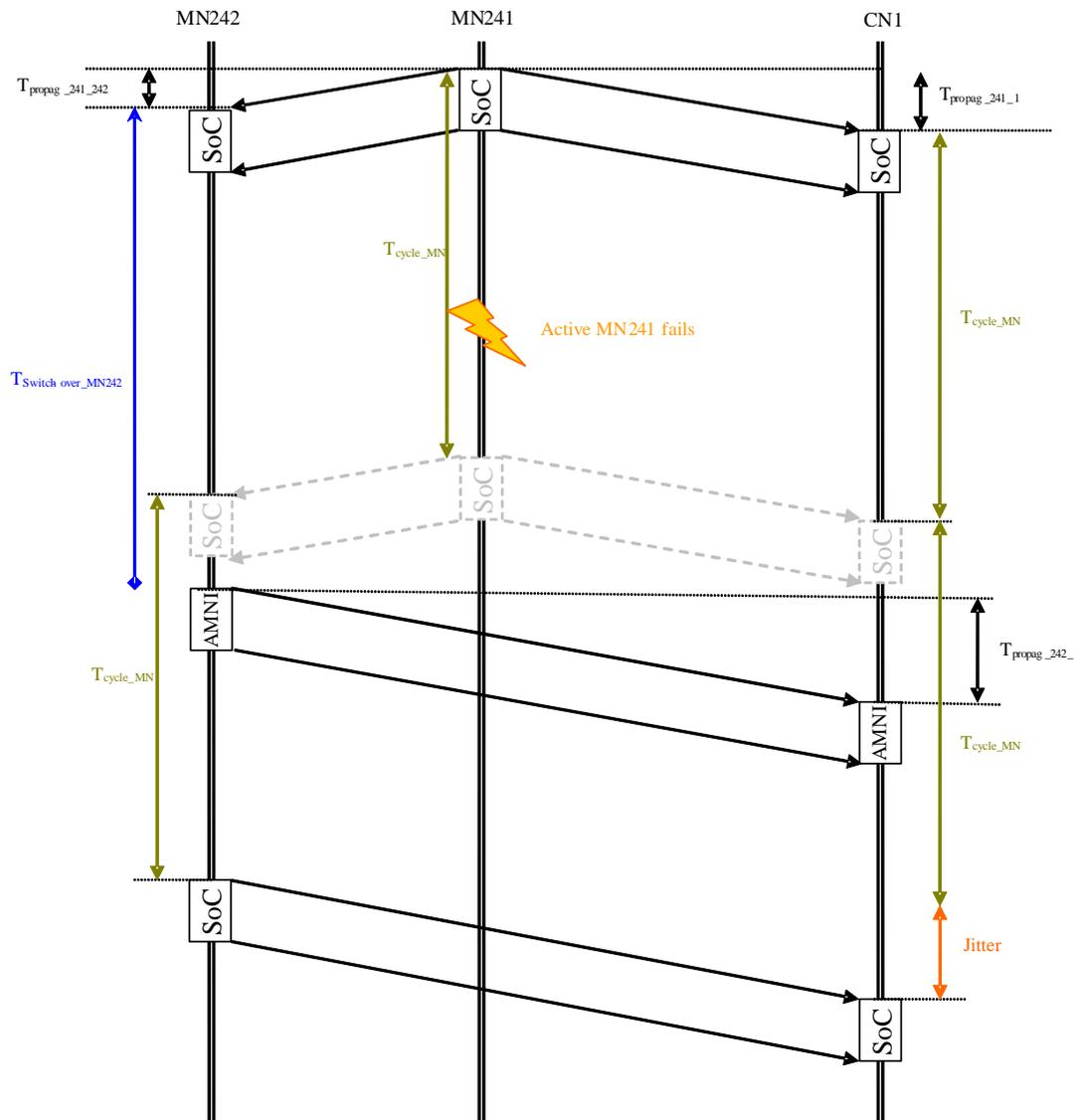
Fig. 22. POWERLINK switch-over timing in isochronous phase
