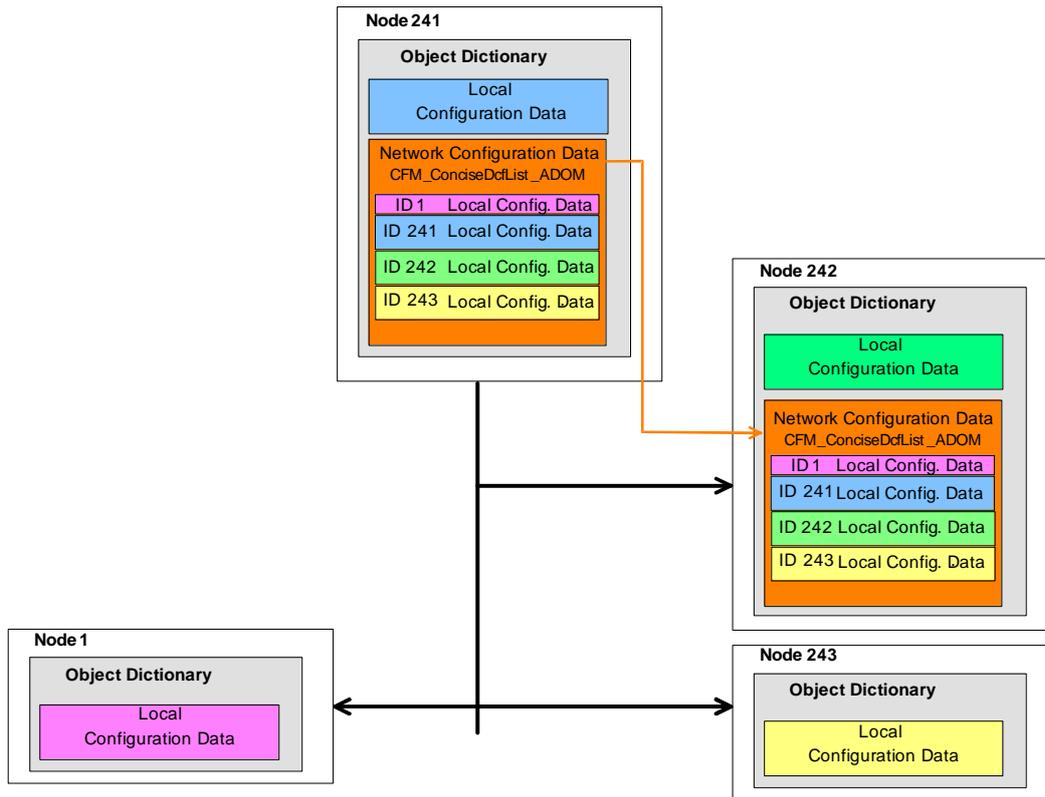
Fig. 13. Update of the network configuration data on RMN 242
