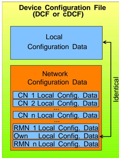
Fig. 9. Setup of the network configuration data
