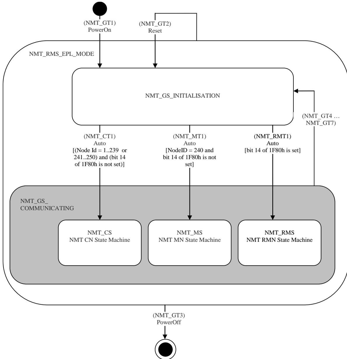
Fig. 14. Common Initialisation of NMT State Machine
