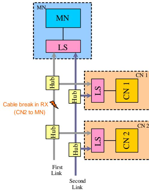
Fig. 4. Example of medium failure
