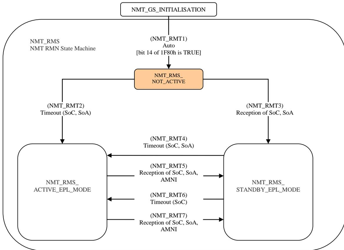
Fig. 15. NMT State Diagram of a RMN
