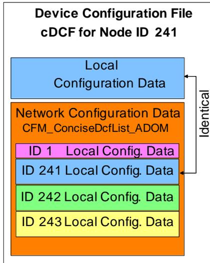
Fig. 11. Example Configuration for RMN 241
