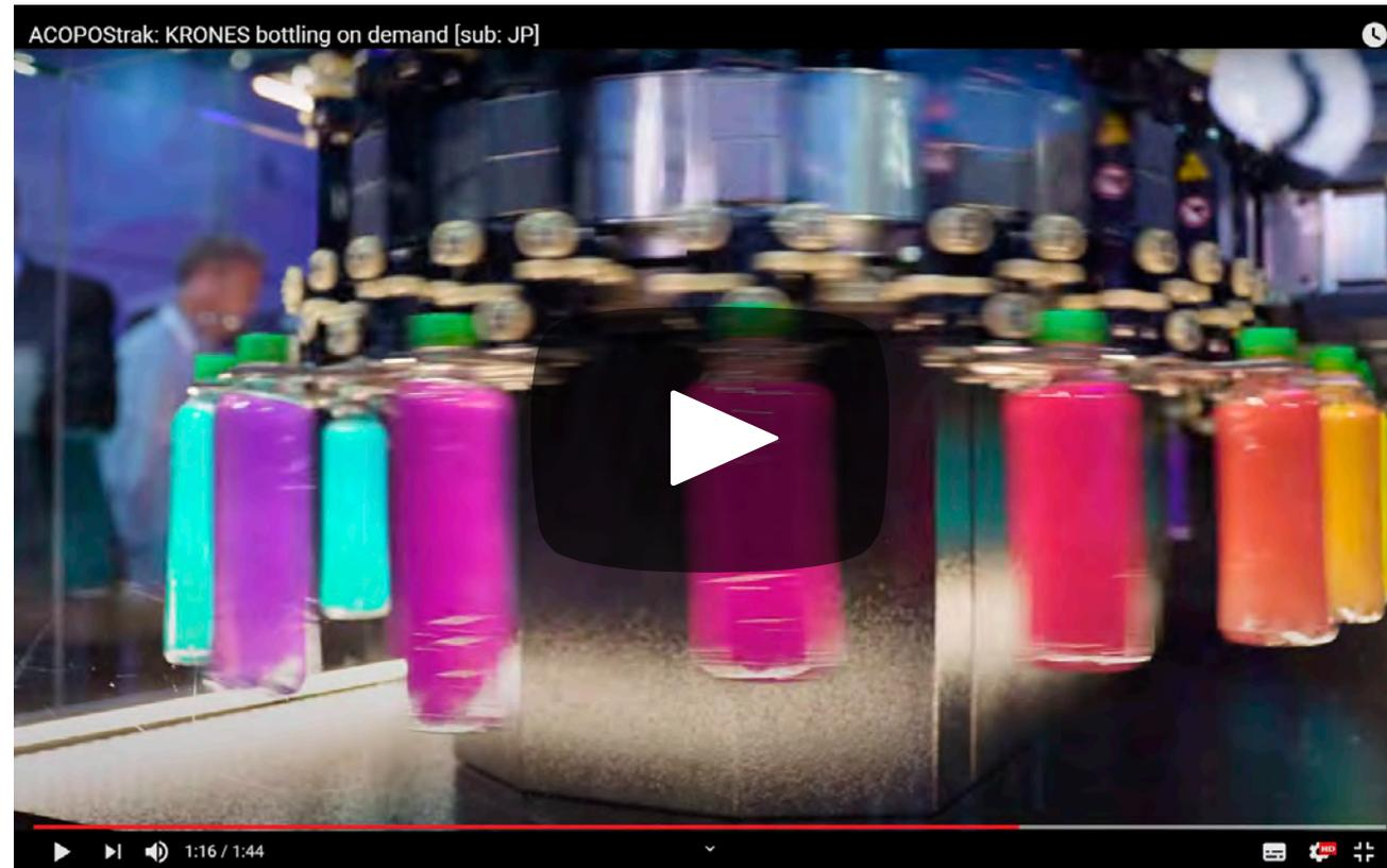
“Bottling on demand” is an adaptive machine concept from Krones capable of batch-size-one formulation, filling, color-coded capping and labeling for beverage lines. It delivers an unprecedented ability to fulfill consumer demand for personalized flavors, portion sizes and even labeling with consumers’ names.
