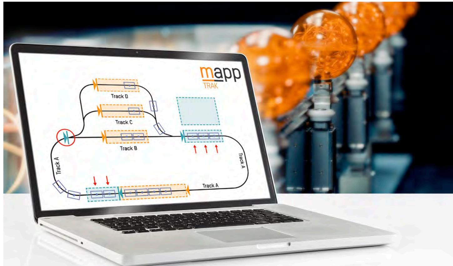
Different shuttle configurations and track layouts can be simulated using a digital twin to optimize line performance before any commitment to capital expenditure is made. Virtual commissioning reduces total cost of engineering and time to market.
